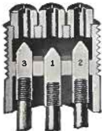
Valves and Valve Seats of "Emergency" Trap—Also Shows Guide Bar for Centering Each Valve.
