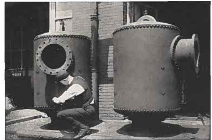
Two 16” “Standard Special” Steel Angle Receiver Oil Separators Furnished to Eliminate Oil and Moisture from Exhaust Steam Before Use in 2,000 KW. Low Pressure Turbines
