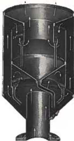
Diagram Showing Flow of Steam Through Head. Baffles and internal condensate drains also are shown.
