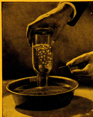
Shows how air is actually sucked up through the water. Compare with Trap above.
